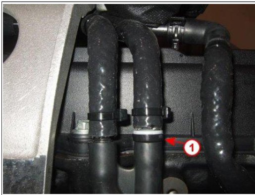
Figure 3 - Upper Check Valve 1. Check Valve - Gray Band Up
