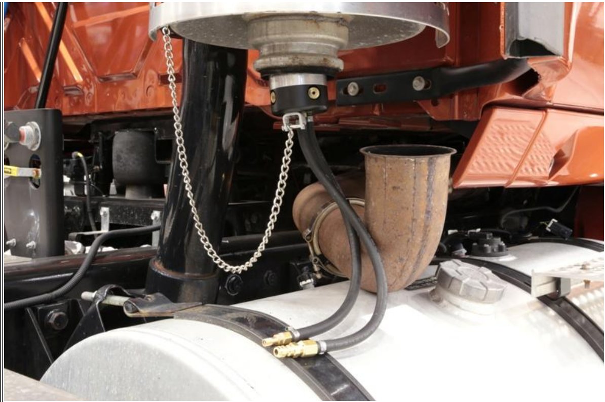
Figure 6: MaxxFace 11/13L vertical exhaust with Powersmoke™ Adapter 2.9 in installed
