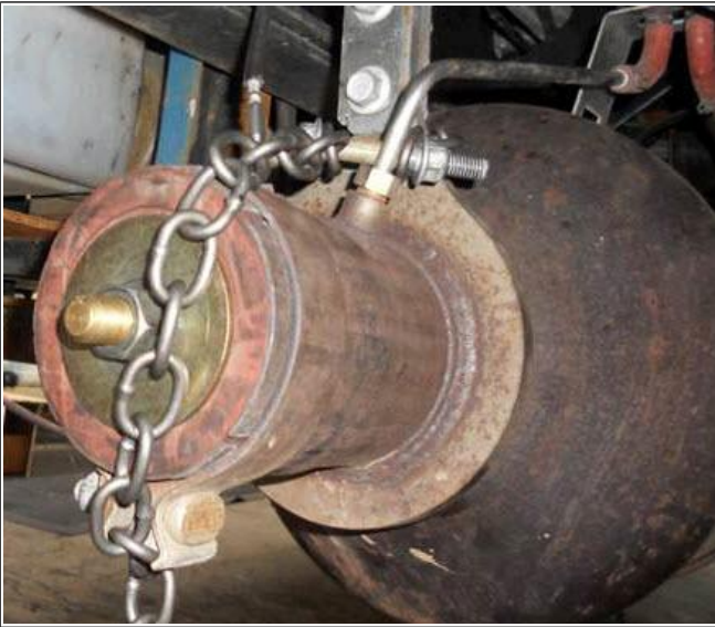
Figure 2: Vertical Restrictor Tool Installation (Tool shown without handle).
