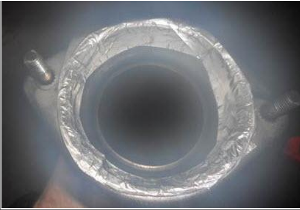
Figure 4: DOC/DPF sealing surface.
