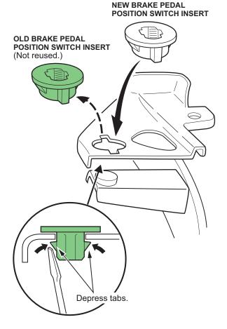
5. Install the new brake pedal position switch insert (white) onto the bracket.
