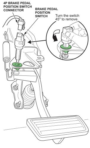
3. Turn the brake pedal position switch counterclockwise 45 degrees and remove it.
