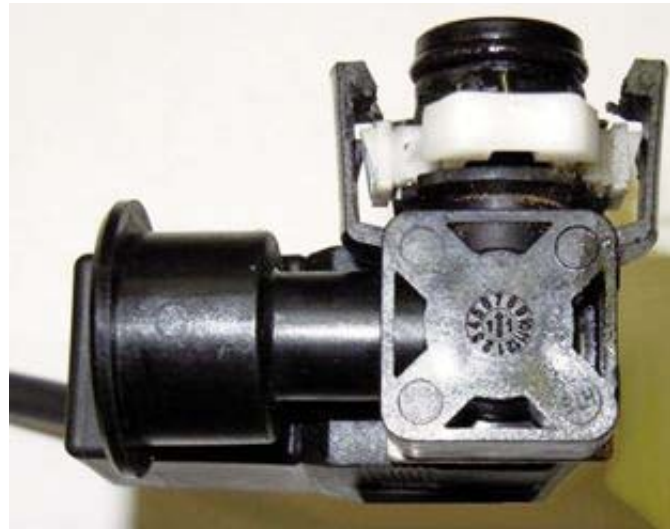
FIGURE 2, 10-WATT SOLENOID VALVE ( 13.5\pm 0.7 \Omega )
