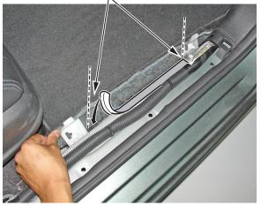
4. Peel back about 50mm (2 inches) of the tape backing starting at the front carpet clip.
