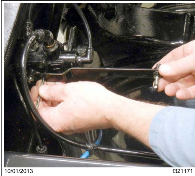
Fig. 1, Inserting a 5/32-inch diameter drill bit or nylon rod to lock the arm in neutral position.
