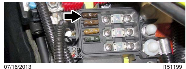
Fig. 15, EPA10 vehicles: 5 amp remote sense fuse, location D in the Powernet Distribution Box (PNDB).
