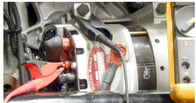
Fig. 14, Clip the DMM positive to the remote sense post and the DMM negative to the alternator body.
