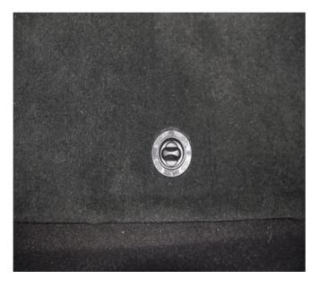
If your vehicle is equipped with a floor mat retaining button(s), hooks(s) or knob(s), make certain the mat is installed correctly and according to the instructions.
