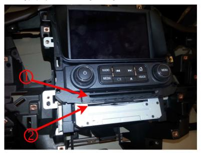
The ICS and multimedia player use two common locating pins (3), as shown below. When the ICS is installed, the two common locating pins (3) may not properly engage into the holes in the back of the ICS, causing the condition.
