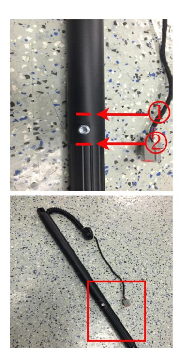
Note: The screw will hold the strut together for removal.
