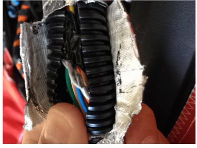
Repair or replace the wiring harness if it is found chafed on the tab of the EGR Valve metal gasket.
