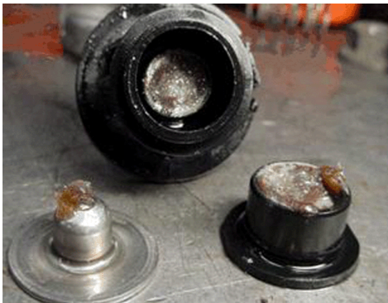
Fuel Pressure Regulator 1 Contaminated With Diesel Exhaust Fluid (DEF)
