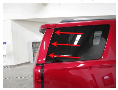
Excessive urethane from the quarter glass installation may not allow the exterior "D" pillar trim to fit properly against the rear quarter glass, as shown below.
