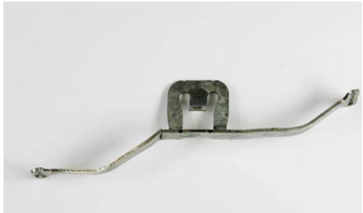
Figure 1. Broken retaining spring.
