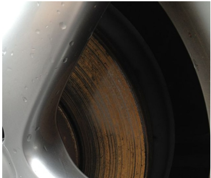
Figure 1. Disc covered with rust.
