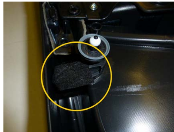
Figure 3. Correct application of felt strip.
