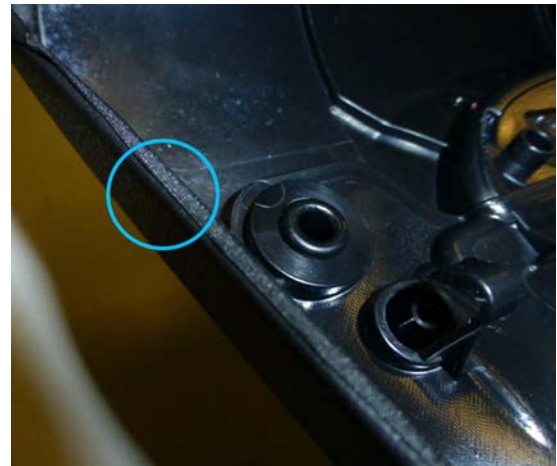
Figure 2. Correct application of textile adhesive tape.
