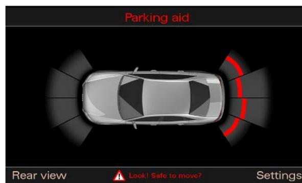
**Figure 1.** Parking aid sensor map with no rear-view camera option in MMI
