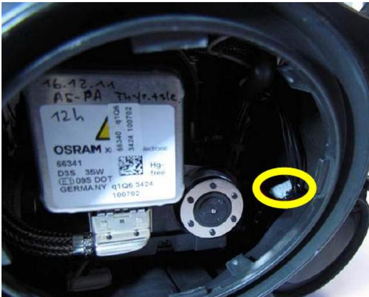
Figure 1. Check this connector on vehicles with PR codes: 8Q3, 8Q5, and 8Q7.
