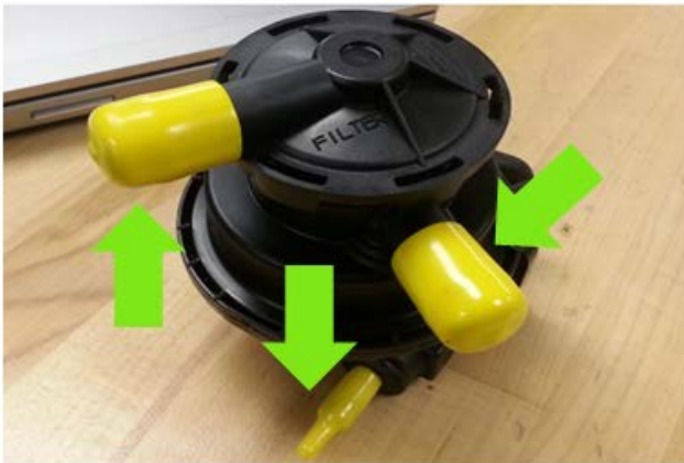
Leak Detection Pump
