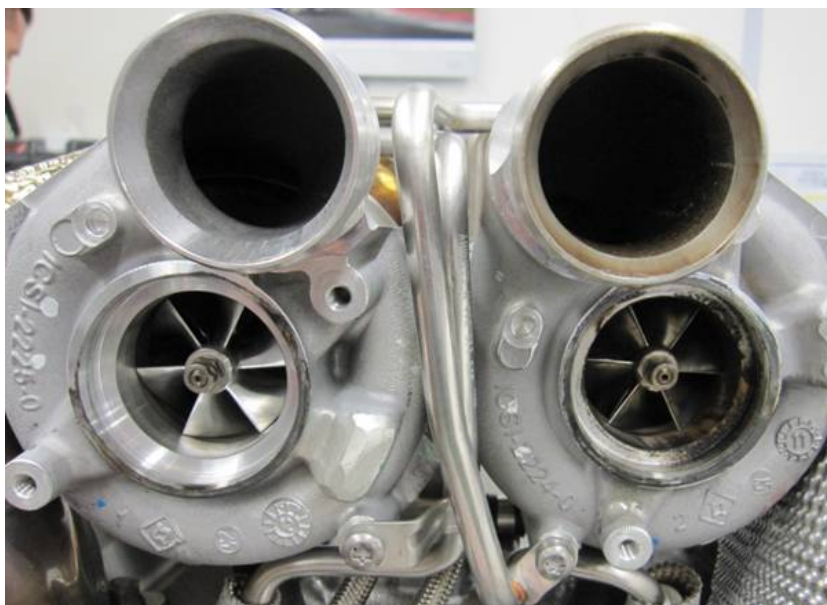
Figure 1. The pipe on the impeller side of the bank 2 turbocharger is discolored due to blow-by gases from the crankcase breather.
