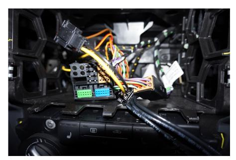
Push the brown connector out of the quad lock. Insert the brown connector from the sound box harness back into the quad lock connector. Insert the brown connector from the factory harness into the black connector in the sound box harness.
