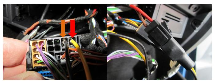
Remove the red and brown wire from the quad lock connector. Insert the red and brown wires into the sound box harness connector. Red to yellow and brown to black (see above). Insert the yellow wire into the position the red wire was removed from and the black in to the position the brown was removed from. (see above).
