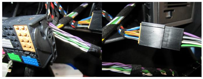
Remove the brown connector from the quad lock connector and insert into the sound box harness connector. Insert the brown connector from the sound box harness back into the quad lock connector.
