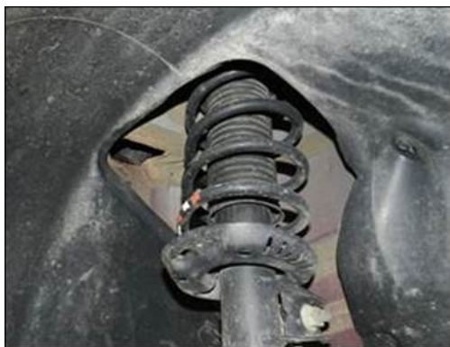
Original wheel liner 561.805.912C.
