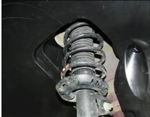
New wheel liner 561.805.912D_9B9 with added material.
