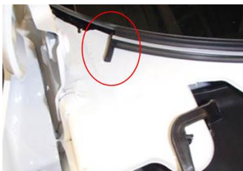
Addition of water deflector 3C0.845.237.
