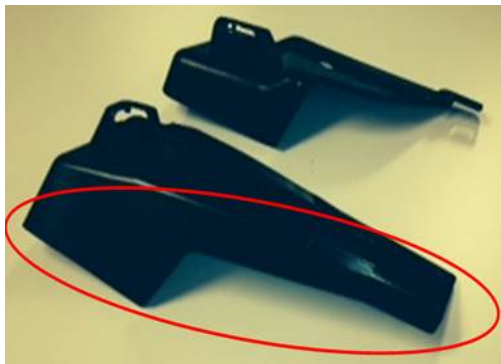
New HVAC air inlet cover 561.815.159C with added material.
