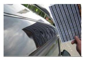
Use the Paint Defect Identifier in photos whenever the condition is difficult to see or assess based on a photo without the tool.
