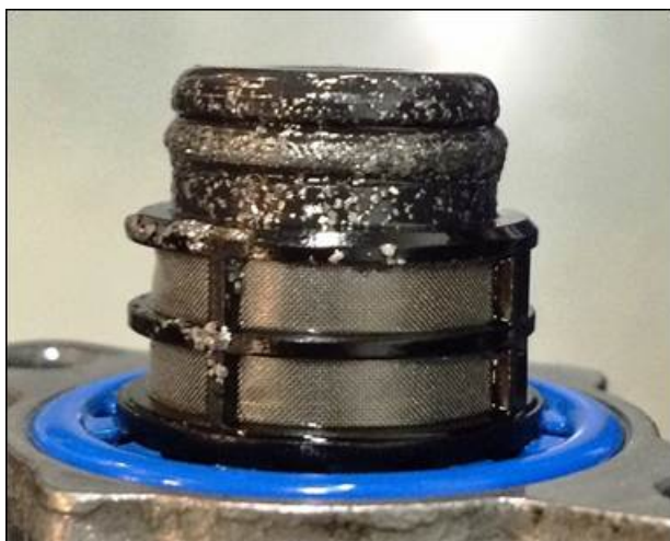
Figure 5. N290 Fuel Metering Valve with Metal Particles
