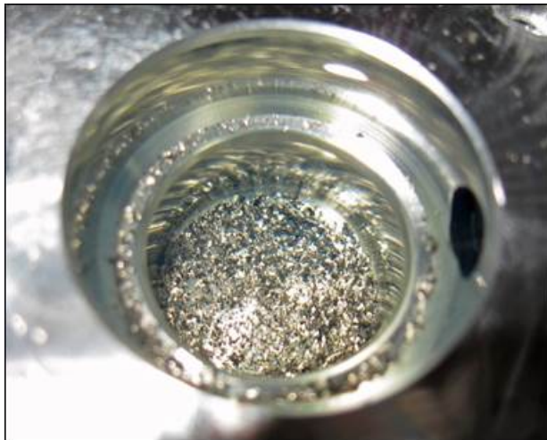
Figure 6. Valve Bore with Metal Particles
