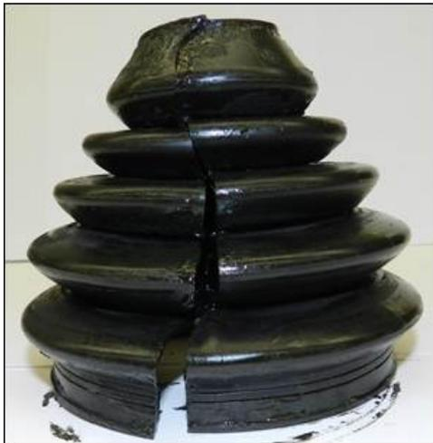
**CV Boots should not be cut or sliced upon removal.**
