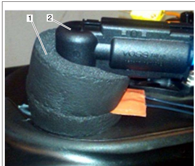
Fig. 1, Cutting the Insulation
