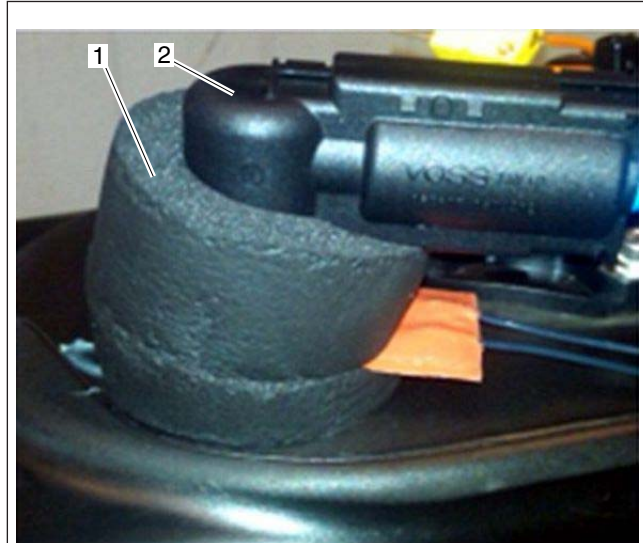
Fig. 3, Installing the Upper Half of the Insulation
