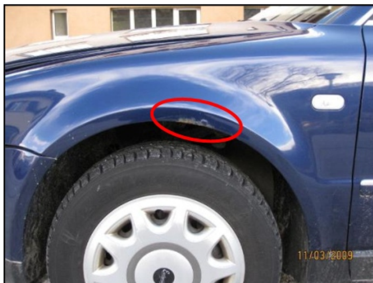
Figure 1 (corrosion on left wheel arch)
