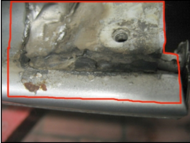
Figure 5 (corroded contact outer rocker panel [side member])
