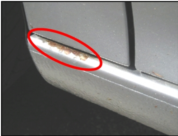
Figure 1 - corrosion in the area of the rocker panel/front fender
