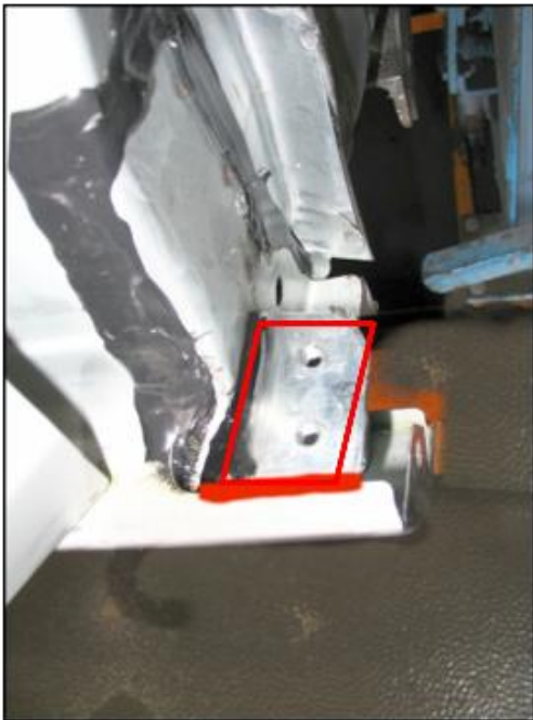
Figure 6 – rocker (side member) during repair
