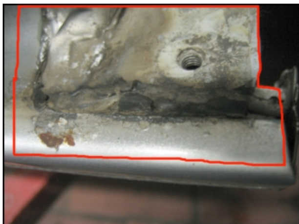
Figure 3 - fender removed (corrosion on the contact surface of the rocker panel [side member])
