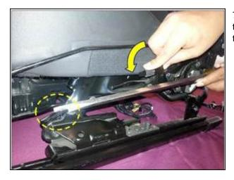
7. Keep the screw driver positioned between the link tab and the track bracket and adjust the seat height to the lowest setting.
