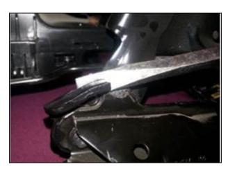
6. Raise the seat back up. Using a large flat head screw driver, place the screw driver blade between the link tab and the track bracket.
