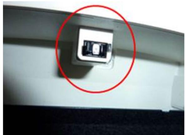
*Figure 1: The sunglass holder spring latch mechanism.*
