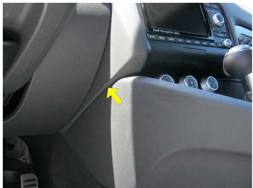
Figure 1. No clearance between the upper and lower sections of the center console.
