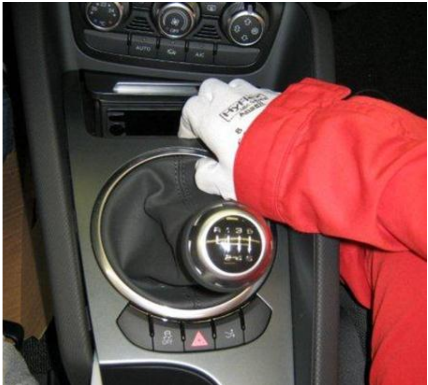
Figure 3. Removing the center console trim.
