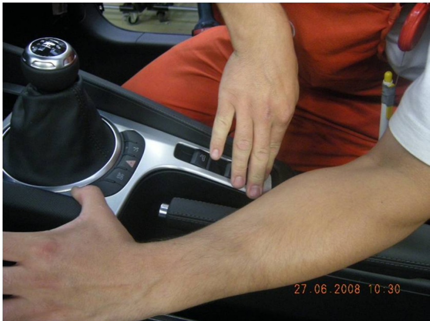
Figure 8. Installation of the center console trim.
