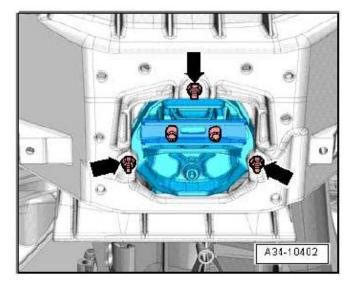
Unscrew bolts <arrows> and detach gearbox support from gearbox together with gearbox mounting.
