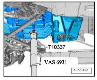
2. Remove bolts <arrows> for tunnel cross member. Tightening torque: 70 Nm
