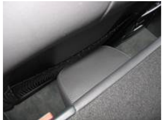
Figure 3: Front seat moved back far enough to make contact with rear seat headrest.
