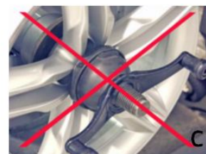
Figure 4. Five-finger style clamping plate (A), wheel properly mounted with a five-finger style clamp (B), and wheel mounted using an incorrect clamping tool/method (C).
