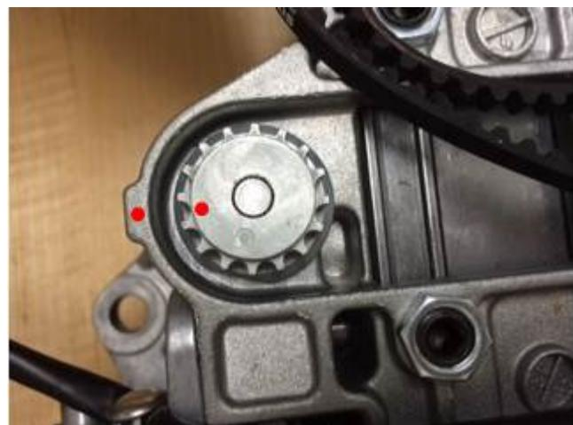
*Figure 5. Marking original gear location.*
