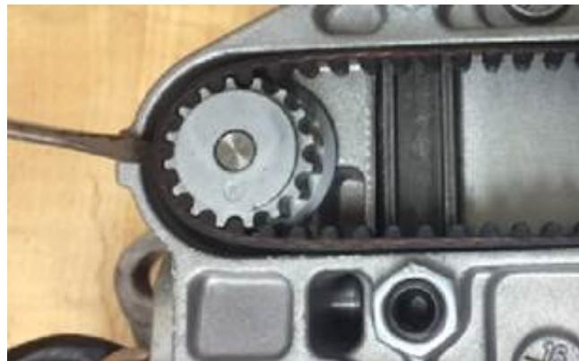
*Figure 4. Remove the gear belt with a fine screwdriver.*
