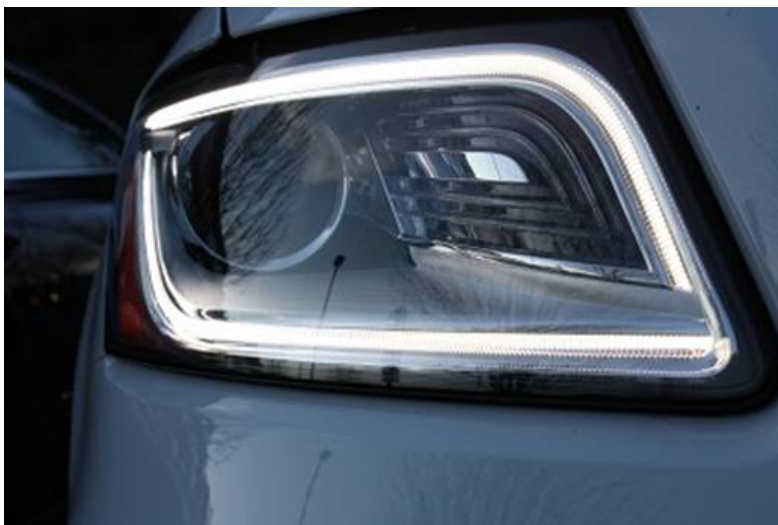
Figure 1. Upper and Lower light pipes illuminated.
