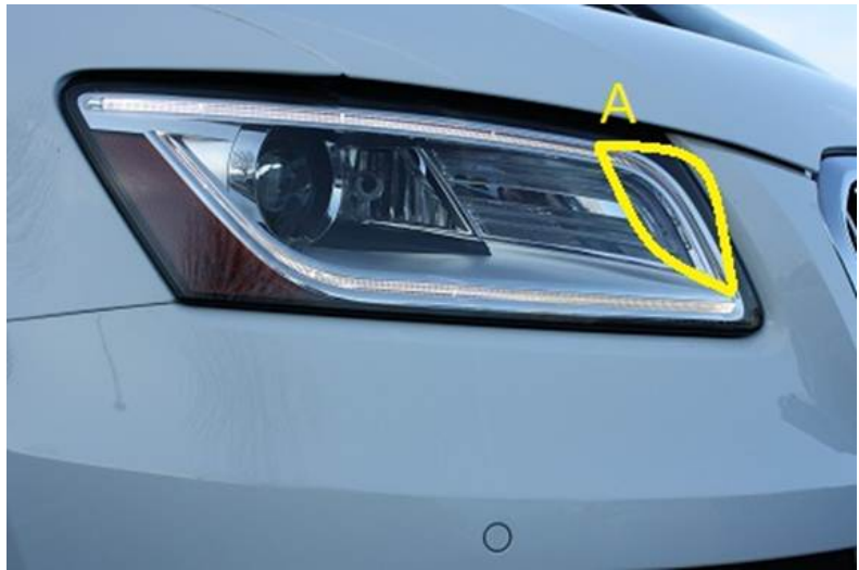
Figure 5. Upper light pipe perceived defect (A).
