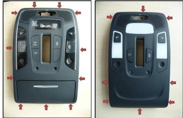
**Figure 2.** Clip location for A6/A7 high-line roof module (left) and for mid-line roof module (right)
