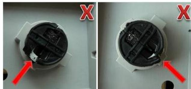
**Figure 4.** Examples of damaged seals
