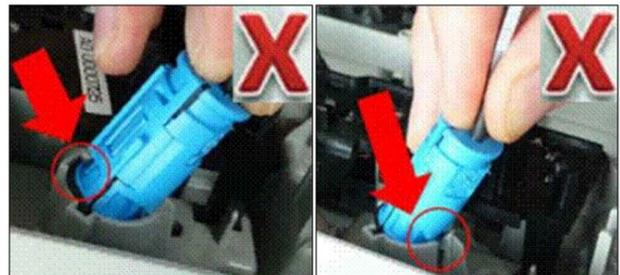
**Figure 6.** Incorrect installation at an angle, showing a pinched seal on the left.
