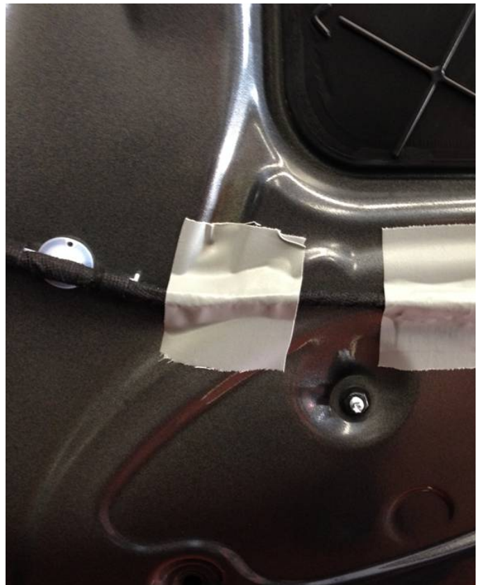
Figure 3. Tape applied to door wiring harness.
