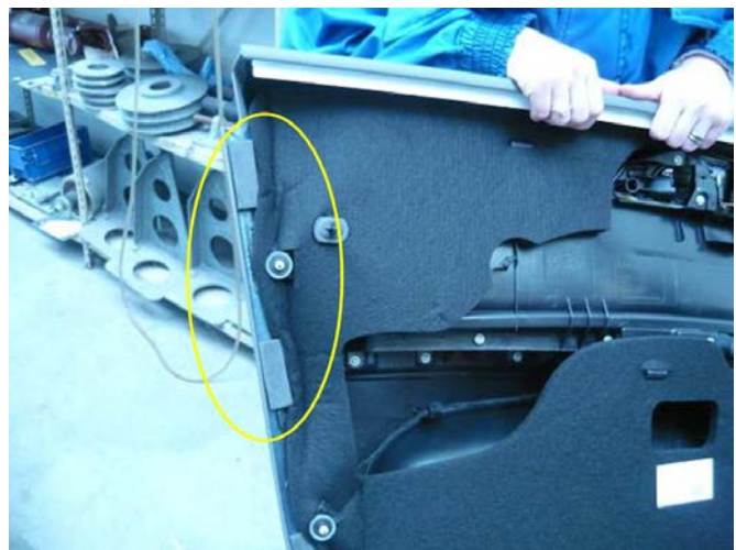
Figure 1. Insulation mat installed around the foam pads.
