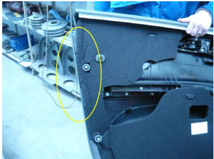
Figure 2. Insulation mat properly installed.
