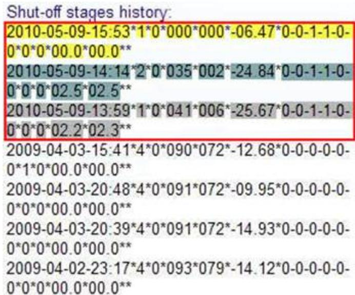
**Figure 7.** Shut-off stages. The reading highlighted in yellow was taken when the battery SOC reached zero, the readings highlighted in blue and in gray were recorded on the same day, before the SOC reached zero.
