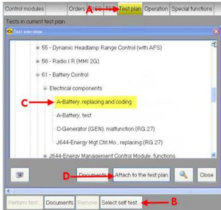
Figure 12. Selecting test plan.
