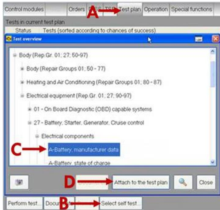
Figure 1. Selecting a test plan in ODIS.
