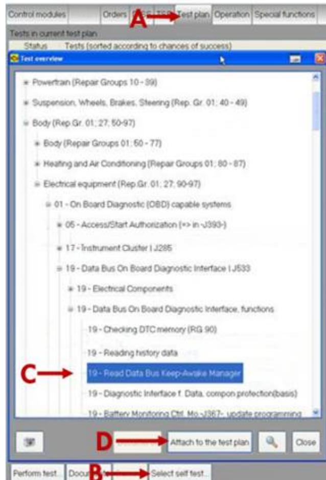
Figure 8. Selecting test plan in ODIS.
