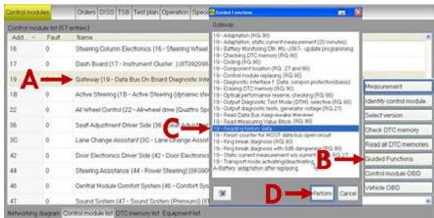
Figure 4. Accessing Reading history data through the Control modules tab.
