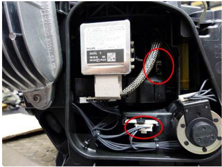
Figure 1. Connectors to be checked.
