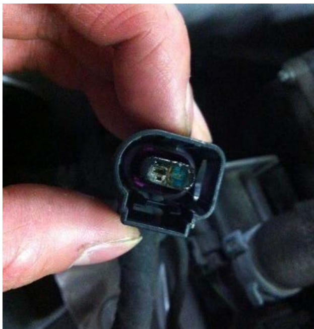
Figure 2. Corrosion formation on the connector pins.
