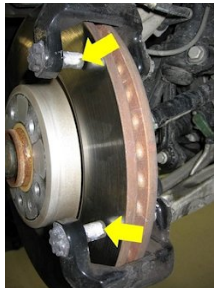
Figure 5. Caliper carrier guide pins with anti-seize lubricant applied where the pads make contact.
