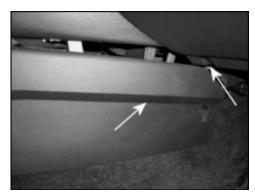
Remove the panels near the foot wells at the passenger side of the console, -arrows-, as shown.
