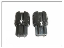
A bushing that fits on the lever may have a broken tab/clip, -arrows-, as shown.
