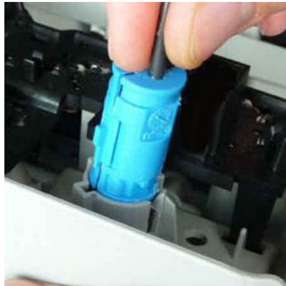
Figure 2. Correct installation angle of microphones.
