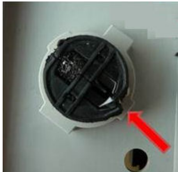
Figure 1. Damaged rubber seal.
