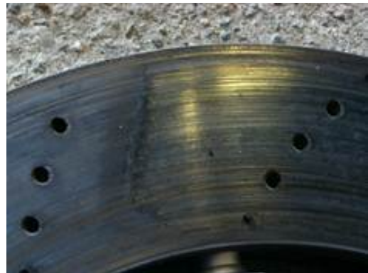
Figure 5. Deposits on the brake disc.
