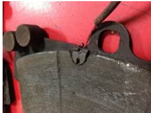
Figure 6. Worn brake pad.
