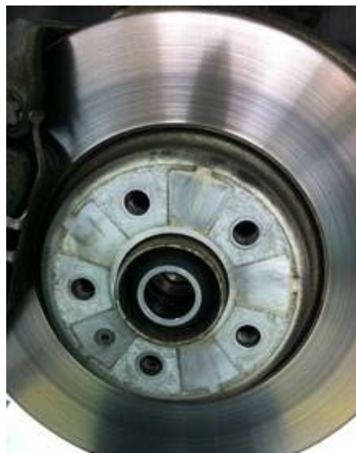
Figure 7: Brake disc with heat marks.
