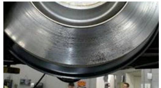
Figure 4. Corrosion marks on the brake disc.
