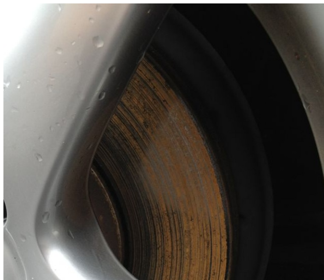
Figure 1. Disc covered with rust.
