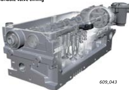
Cylinder head with variable valve timing
