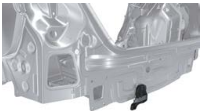
Access/Start System Antenna in Rear Bumper R136.
